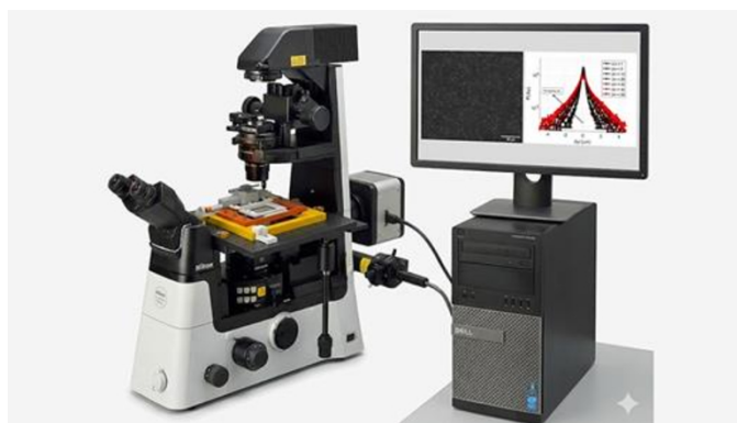
Schematic view of ShearView platform integrated on an inverted optical microscope. The compact linear rheometer is mounted around the sample stage and coupled to a computer for real-time acquisition and control.
