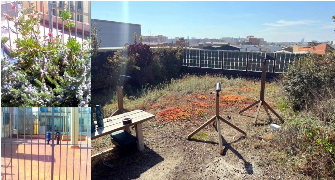
Figure 2. Location of IR sensors in two of the studied green roofs. The two left images are from GR1 roof and the right image is from GR2 (another green roof for which we don't show results here). The top-left image shows the visual field of the IR sensor measuring the temperature of a parterre with vegetation. The bottom-left image shows two IR sensors, one pointing at a vegetation surface and the other at a neighbouring roof with ceramic roof tiles, the same system that GR1 had before the green solution was implemented. In GR2 we have set up 3 IR cameras, one pointing at high vegetation (right), another at low vegetation (left) and another at a bare-substrate zone (centre).
