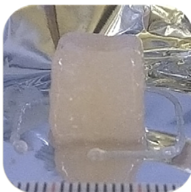
Fig. 1. 3D printed gel cube from a mixture of low acyl gellan gum and tamarind seed gum containing 5 wt% pea protein isolate.
